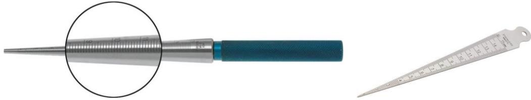
Tool for measuring the gap: Bore gauge or tapered measuring wedge; due to manufacturing inaccuracies, the gap may not be the same all the way around. Ensure there is no contact between the rotating impeller and the fixed inlet nozzle at any point.
